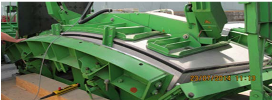
Figure 13: Demoulding of segment.
