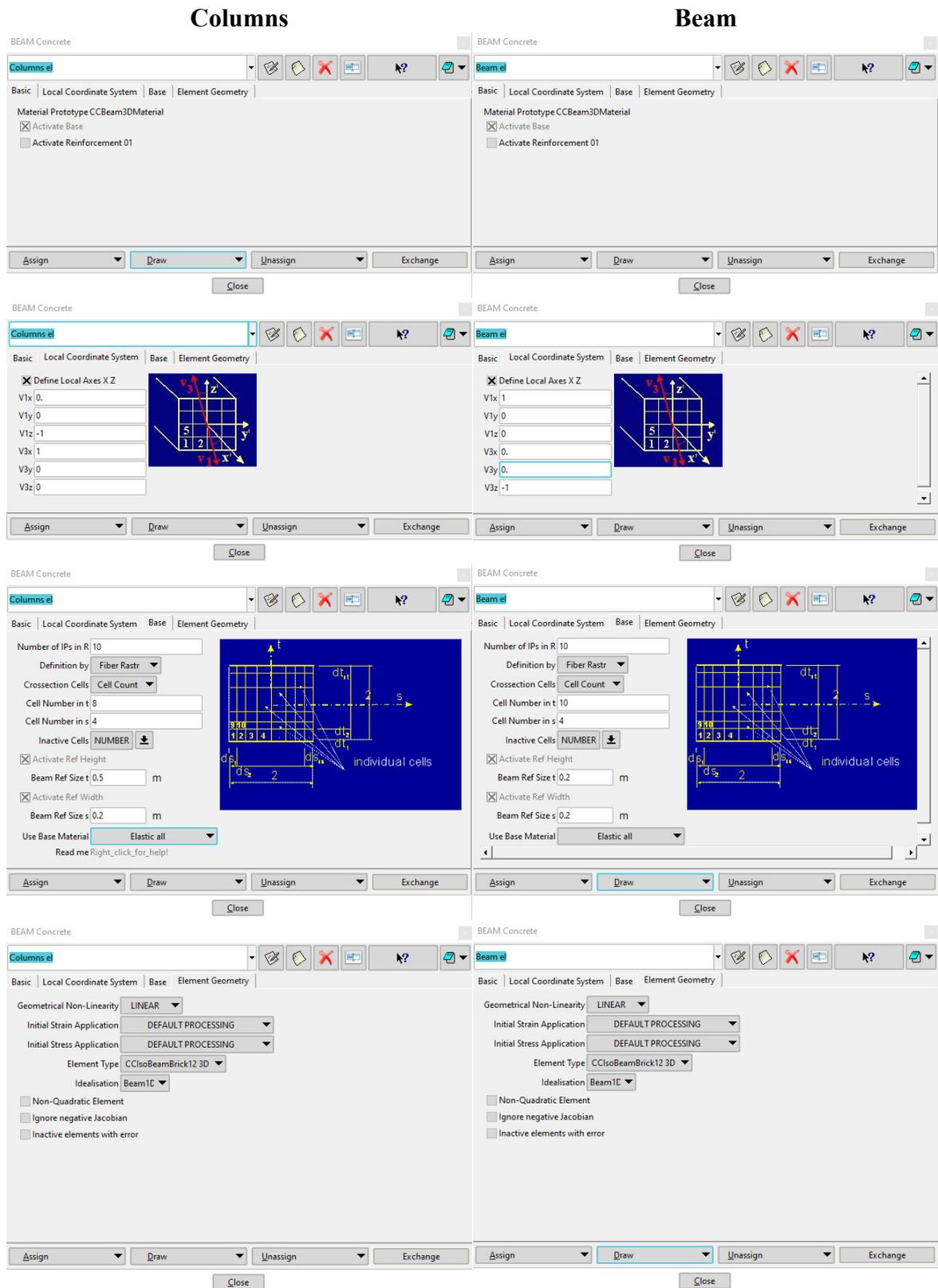
Figure 2-48 Definition of 1D BEAM elements for beam and columns.
