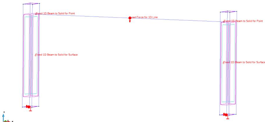
**Figure 2-53 Model combining line geometry (1D beam) and volumes (3D solids).**
