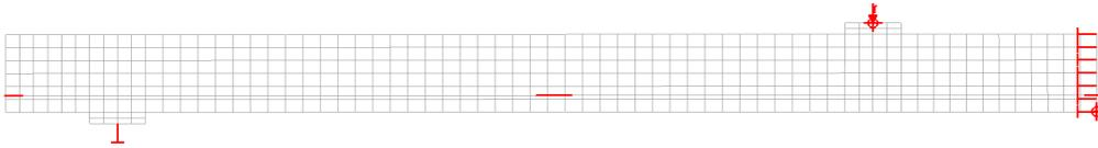
**Figure 3-3: Two-dimensional finite element model.**
