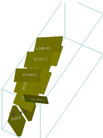
Fig. 5-43 Crack width label inside of structure. Fig. 5-44 Cracks in integration points.
